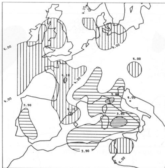
Figure 3.12 Regional phase velocities of Rayleigh waves at a period of 50 sec. Vertically hatched areas are faster than average (3.95 km/sec), horizontal hatched areas are slower. (Wielandt and Mueller, with permission)
